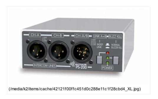
Case will be 1U high x 1/4 rack wide -110 mm- and about 150 mm deep. Rear panel includes an IEC connector w/fuse holder and a rocker mains switch. Front panel includes one XLR 3 male for CHA, one XLR 3 male for CHB, one XLR 5 male for A/B channels, one A/B link switch with led indicator and a BUZZer Kill sw itch w ith led indicator to allow the use in quiet shows as in theatres.
