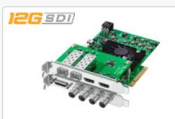
**DeckLink 4K Extreme 12G** Capture and playback 12G-SDI in SD, HD, Ultra HD and 4K DCI up to 4096 x 2160 60p in 10-bit YUV or 12-bit RGB!
