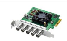
**DeckLink Duo 2** PCIe capture and playback card with 4 independent channels for SD and HD up to 1080p60.
