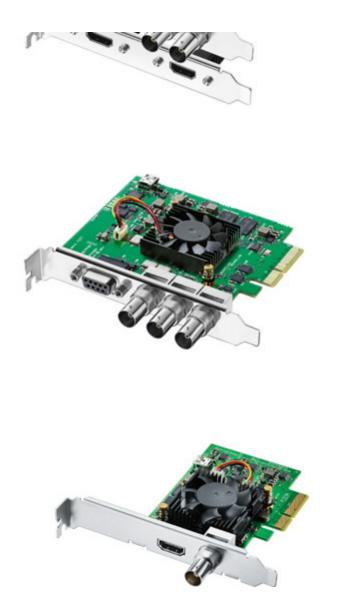
switchable to 6 ch out, black burst and tri-sync reference input, RS-422 deck control connections, keying in SD and a hardware down converter. Perform editing, paint and broadcast design and more with the ultimate future proof design!
