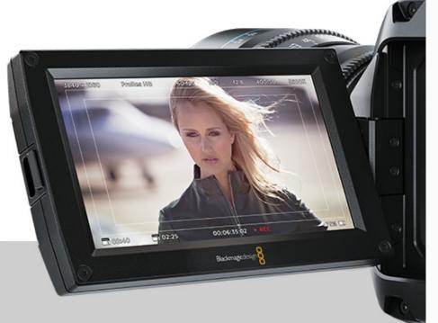
The high resolution 5 inch fold out monitor includes a touchscreen so you get easy access to the revolutionary URSA camera interface. All of your settings, controls and monitoring tools are at your fingertips. That means you don't have to hunt through confusing menus to make changes. You can see and change all camera settings, view timecode, histograms for checking levels, audio levels and a focus peaking indicator for checking focus!
