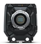
User upgradeable, full size digital film camera with film industry PL lens mount and 4K Super 35 sensor with global shutter, 12G-SDI, built in 10" monitor, dual CFast recorders, scopes, audio meters and more!
