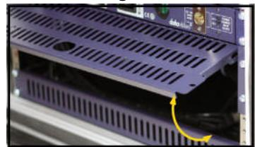
Easy access to internal cable loom and storage for additional cabling during transport is made easy with the quick release pivoting back panel
