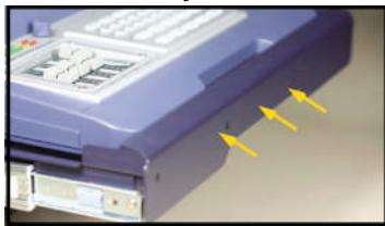
Securing the SE-500 during transport and operation, while maintaining access to headphone and microphone
