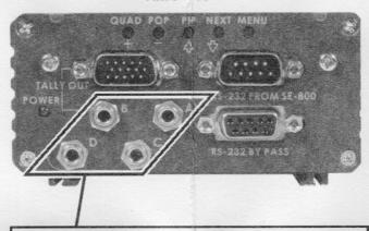
Connect the TD-1 to the RMC 140 Tally Light Output 3.5mm Jack Sockets, via the CB-1 cable.
