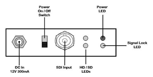
**HD / SD LEDs -** Once a signal has been detected the appropriate LED will light to indicate format. **Signal Lock LED** - The LED will light up when a SDI signal is detected.
