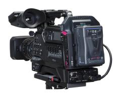
The new and improved CW-7 wireless HD-SDI/SD-SDI transmission system now offers superior image quality, even more compatible video formats and up to 50m range with zero delay. The CW-7 has increased transmission power on all 4 channels and now features DFS (Dynamic Frequency Selection) for use in a wider range of indoor and outdoor applications, detecting official radio frequencies used within the 5GHz band and automatically switching to a safer and less congested channel.
