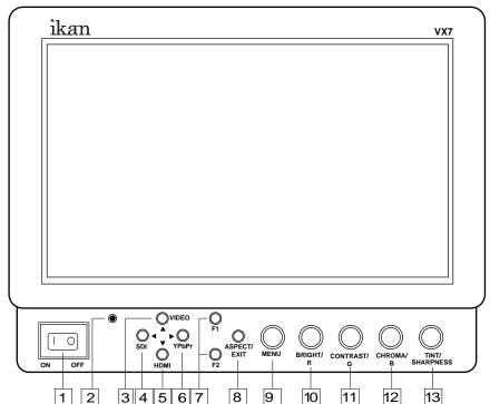
User programmable function buttons. For quick access, the user may program the F1 and F2 buttons to enable frequently accessed monitor features. Via the main monitor configuration menu, either button may be assigned to perform the following functions: Window 1, Window 2, HV delay, Blue Gun, and Pixel to Pixel, .
