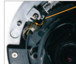
When three metal levers are turned clockwise, springs work automatically to fix the unit firmly into the ceiling.
