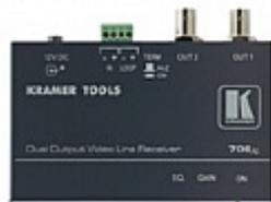
The 705xl and 706xl are a twisted pair transmitter and receiver for composite video signals. The 705xl converts a composite video signal to two twisted pair signals and the 706xl receiver converts the twisted pair signals back into two composite video signals.
