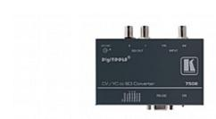
The 7508 is a multi-format converter for composite video or s-Video (Y/C) signals. It converts either PAL, SECAM, and NTSC composite or s-Video (Y/C) signals into two SDI video (SMPTE 259M) outputs simultaneously.
