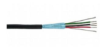
Kramer's BC-2T is a high-quality, dual shielded pair cable designed for routing balanced stereo mic or line level audio signals in commercial or residential AV systems.
