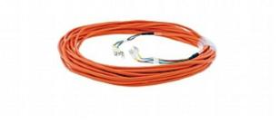
Kramer's 4LC fiber optic cables are constructed of four color coded multi-mode 50/125um simplex cables of 2.0mm (0.079in) diameter each, contained in a round overall orange jacket. They are intended primarily as companion to various Kramer detachable transmitter/receiver sets.
