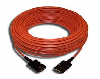
Kramer's new all DVI cable system is constructed of high-performance hybrid cable containing fiber optic and copper wires terminated with DVI-D connectors on each end. They are designed to transmit DVI-D signals extremely long distances with pristine digital image quality video with the copper cable carrying additional data required for HDCP compliance.
