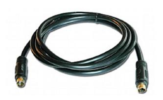
Kramer's SM series cables are high performance s-Video (Y/C) cables with molded 4-pin mini DIN connectors at each end. Luminance and chrominance signals are carried on separate internal coaxes for superior quality over composite video.
