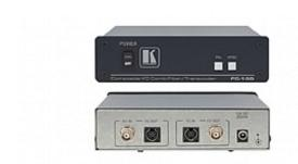
The FC-10D is a highperformance bidirectional transcoder for composite and s-Video (Y/C) signals. The unit simultaneously converts a composite video input to an s-Video output through a digital comb filter, and an s-Video (Y/C) input to a composite video output.
