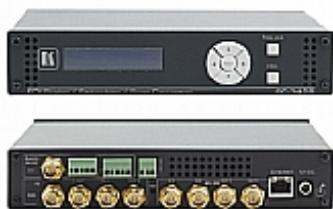
The FC-340S is a broadcast-quality video scaler and audio embedder/de-embedder for digital signals up to 3G HD-SDI. The unit inputs SDI and AES/3id signals and simultaneously outputs two SDI and composite video signals while the audio embedded in the SDI input signal is output to both AES/3id and balanced stereo audio outputs.
