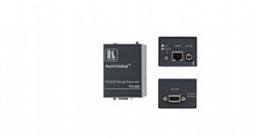
The FC-50 is a bidirectional range extender for RS-232 signals. The unit accepts an RS-232 signal that is converted to a twisted pair signal and sent to a second FC-50 that converts the twisted pair signal back into an RS-232 signal.
