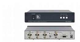
The FC-7501 is a format converter for composite video, s-Video or component video (YUV) signals. It converts either PAL, SECAM, and NTSC composite video, s-Video, or component (YUV) signals into 2 SDI (SMPTE 259) signals simultaneously.
