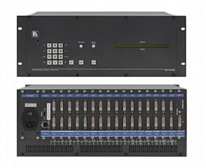
The VS-1616D is a high-performance matrix switcher chassis for AV signals. The unit is modular and populated from 2x2 to 16x16 in increments of two inputs and/or two outputs. The chassis includes a power supply, control module and a test module that can monitor and test any input and output in the matrix.
