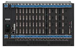
The VS-3232DN is a high-performance matrix switcher chassis for DVI & HDMI signals. The unit is modular and populated from 4x4 to 32x32 in increments of four inputs and/or four outputs. The chassis includes one power supply but can also accept a second redundant power supply (sold separately), a control module and a test module that monitors and tests any input and output in the matrix.
