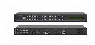
The KADS-100 (Kramer Audio Distribution System) is a master audio controller for use with multiple, remote, active KADS-1 and KADS-2 speakers. It features eight unbalanced mono audio inputs, one S/PDIF digital stereo audio input, and one USB connector for mass-storage devices. RS-232 data and commands flow bidirectionally allowing remote status requests and control of the speakers.
