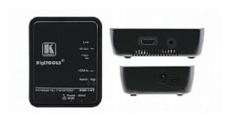
The KW-14T is a high-definition, wireless, HDMI transmitter for indoor use. Up to four KW-14R receivers can receive from one KW-14T transmitter and up to three KW-14T transmitters can be paired with one KW-14R receiver. The KW-14T and KW-14R pair comes pre-associated.
