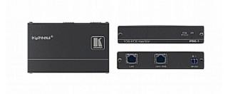
The PSE-1 provides power remotely over Ethernet to any device capable of acting as a PoE acceptor (for example, a wallplate, where it may be difficult to connect an external power supply). This allows a single HDBT LAN cable to provide both data and electrical power to compatible devices.
