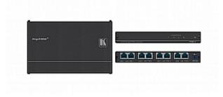
The PSE-4 is a four-way PoE (Power-over-Ethernet) injector that supports 4K UHD video. The unit provides power remotely over Ethernet to up to four devices capable of acting as PoE acceptors, (for example, the DIP-20, where it might be difficult to connect an external power supply). This allows a single HDBT LAN cable to provide both data and electrical power to compatible devices.
