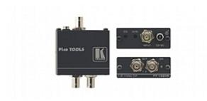
The PT-102VN is a distribution amplifier for composite video or SDI signals. It takes one input, provides correct buffering and isolation and distributes the signal to two identical outputs.
