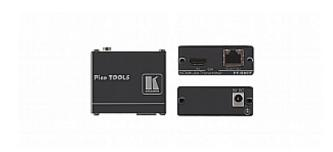
The PT-580T is a 4K resolution, HDBaseT twisted pair transmitter for HDMI signals. The unit inputs an HDMI signal that it converts to a twisted pair signal. An HDBaseT receiver (for example the TP-580R or WP-580R) converts the twisted pair signal back into an HDMI signal and together they form a transmitter receiver pair.
