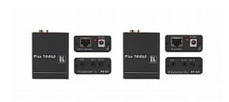
The PT-5T and PT-5R are a twisted pair transmitter and receiver for infrared signals. The units control up to five devices via their own remote control IR transmitters at distances of up to 250m (820ft) over twisted pair cable.
