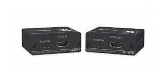
PT-871/2-KIT is a high-performance, long-reach DGKat™ 2.0 extender kit for 4K@60Hz (4:4:4) HDR HDMI 2.0 and HDCP 2.2 signals and 2-way powering over twisted pair. The PT-871 transmitter converts the HDMI input signal into a DGKat™ 2.0 signal. The PT-872 receiver converts the transmitted DGKat™ 2.0 signal into an HDMI signal. PT-871/2-KIT extends video signals to up to 40m (130ft) over Kramer shielded cables at up to 4K@60Hz (4:4:4) 24bpp video resolution
