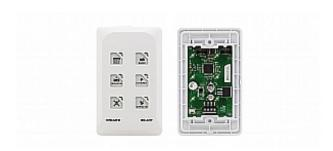
The RC-43T is a 6-button auxiliary control panel that works as a remote control panel for master room controllers such as the SL-1 in classrooms, boardrooms or auditoriums. The RC-43T buttons are touch-sensitive and give press confirmation using their LEDs.
