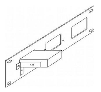
19-inch rack adapter for mounting 3 desktop models into a 2U rack space.
