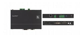
The SID-X1 is a DGKat™ twisted pair transmitter and step-in commander for computer graphics video, HDMI, DVI, DisplayPort and unbalanced stereo audio signals. The unit includes a "Step-In" button that allows the local source to be routed as the active source on the main display through the main switcher.
