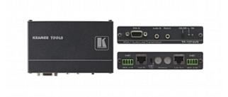
The TP-107AVR is a twisted pair transmitter for computer graphics video signals with resolutions exceeding UXGA and stereo audio signals. The unit switches between a twisted pair input and a computer graphic video input with stereo audio. It outputs to a single twisted pair that is sent to a compatible receiver.
