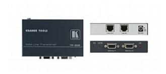
The TP-202 is a twisted pair branching receiver for computer graphics video signals with resolutions from VGA up to UXGA and higher or HDTV signals. It takes a twisted pair signal and converts it into a computer graphics video signal or HDTV signal available on two 15-pin HD outputs, and simultaneously re-transmits the original twisted pair signal to another compatible receiver.
