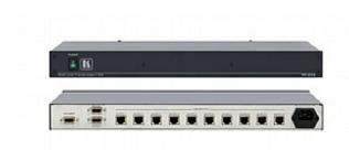
The TP-210 is a highperformance distribution amplifier for computer graphics video signals with resolutions ranging from VGA through UXGA and higher. It takes one input and provides 10 twisted pair outputs plus two computer graphics video outputs on 15-pin HD connectors for local monitoring.
