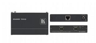
The TP-330FW is a twisted pair range extender/hub for FireWire® (IEEE 1394) signals. When used as a pair, one converts a FireWire® signal into a twisted pair signal and the other converts the twisted pair back to a FireWire® signal and simultaneously outputs the twisted pair signal to two FireWire® ports.
