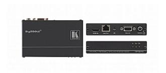
The TP-573 is a DGKat<sup>™</sup> twisted pair transmitter for HDMI, bidirectional RS-232 and infrared signals. The TP-573 converts the input signals to a twisted pair signal and the TP-574 converts it back to HDMI, RS-232 and infrared signals.
