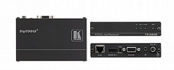
TP-580R is a high-performance, long-reach HDBaseT receiver for 4K60Hz (4:2:0) HDMI, RS-232 and IR signals over twisted pair. It extends video signals to up to 40m (130ft) over CAT copper cables at up to 4K@60Hz (4:2:0) 24bpp video resolution and provides even further reach for lower HD video resolutions.
