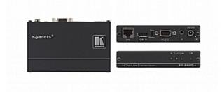
The TP-580TXR is an extended range, HDBaseT twisted pair transmitter for HDMI, bidirectional RS-232 and IR signals. The TP-580TXR inputs HDMI, RS-232, and IR signals and converts them into an HDBaseT twisted pair signal that it transmits to a TP-580RXR receiver.
