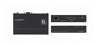
TP-580Txr is a high-performance, extended-reach HDBaseT transmitter for 4K60Hz (4:2:0) HDMI, RS-232 and IR signals over twisted pair. The TP-580Txr converts all input signals into the transmitted HDBaseT signal. It extends video signals to up to 100m (330ft) over CAT copper cables at up to 4K@60Hz (4:2:0) 24bpp video resolution and provides even further reach for lower HD video resolutions.
