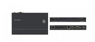
The TP-582T is a high-quality twisted pair transmitter for HDMI, Ethernet 100BaseT, bidirectional RS-232 and IR signals. The TP-582T selects one of two HDMI inputs, and converts it with the Ethernet 100BaseT, RS-232 and IR input signals to a twisted pair signal. The TP-582R converts the twisted pair signal back to Ethernet 100BaseT, RS-232, IR and two HDMI outputs, and de-embeds the audio to S/PDIF and TOSLINK® audio outputs.
