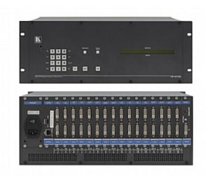
The VS-1616D is a high-performance matrix switcher chassis for AV signals. The unit is modular and populated from 2x2 to 16x16 in increments of two inputs and/or two outputs. The chassis includes a power supply, control module and a test module that can monitor and test any input and output in the matrix.
