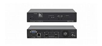
The VM-114H is a switcher/distribution amplifier for HDMI and DGKat™ twisted pair signals. It reclocks and equalizes one of two selectable input signals and distributes it to four identical HDMI outputs.
