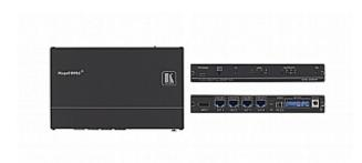
The VM-4HDT is a high-quality 1:4 4K UHD HDMI to HDBT distribution amplifier that takes one HDMI input, equalizes and reclocks the signal and distributes it to four identical HDBT outputs. The VM-4HDT distributes signals having resolutions of up to [email protected] (4:2:0) UHD including WUXGA and 1080p.
