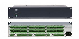
The VM-54A is a highperformance distribution amplifier for balanced stereo signals. It can also be configured as three 1:18 distribution amplifiers for balanced stereo audio.
