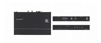
The VP-425 is a high-performance digital scaler for computer graphics video and component HDTV signals. It up- or down-scales the input and embeds the stereo audio into the non-HDCP encrypted HDMI output.
