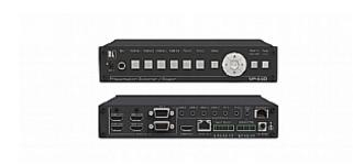
The VP-440 is a high-performance presentation scaler/switcher with four HDMI and two computer graphics (VGA) inputs. The unit scales the video, embeds the audio and outputs the signal to an HDMI output and an HDBaseT output simultaneously. The unit includes analog and embedded audio inputs and outputs.
