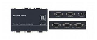
The VP-250, VP-350 and VP-450 are high-performance distribution amplifiers for computer graphics video signals with resolutions ranging from VGA through UXGA and higher. They take one input, provide correct buffering and isolation, and distribute the signal to two, three and four identical outputs.
