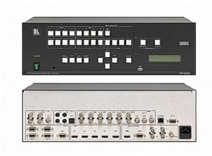
The VP-725N is a presentation scaler/switcher with multiple signal format sections. The unit has five independent 4x1 video sections: composite, s-Video (Y/C), component (YUV), computer graphics, and HDMI, plus a single USB input. It also up- or down-scales any video input to a selectable graphics or HDTV output resolution. FTB<sup>TM</sup> (fade-thru-black) switching technology provides glitch-free switching between sources.
